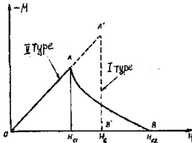
*Fig. 1.7. Curves of magnetization of the of the I and II type superconductors having a form of the long cylinder in a longitudinal field*
