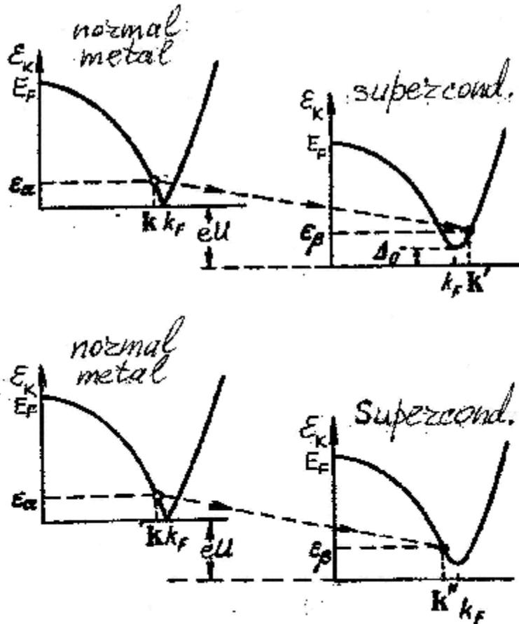
Fig. 1.10. One-particle tunneling between a normal metal and a superconductor.
