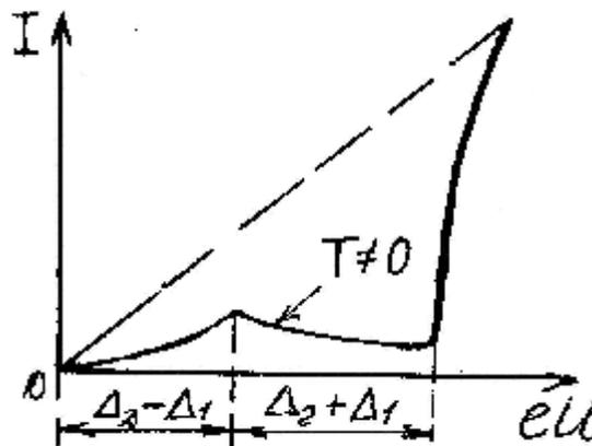
Fig. 1.13. Tunneling between two superconductors.
