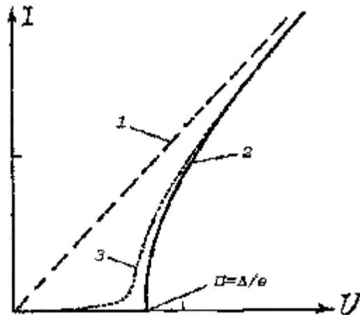
Fig. 1.12. Volt-Ampere characteristics of tunnel contacts.
