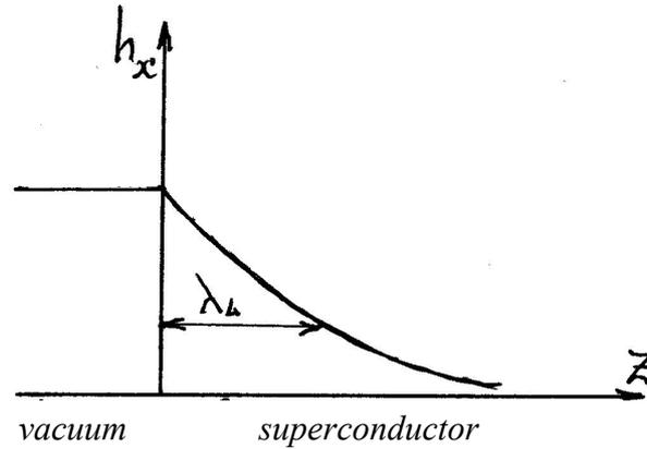
Fig.2.4. Penetration of a weak magnetic field into the superconductor.
