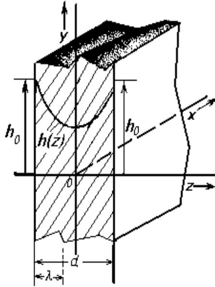
Figure 2.5. The distribution of the magnetic field inside the thin superconducting film.
