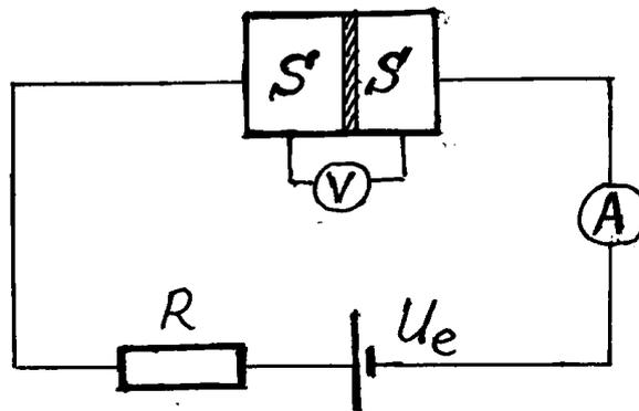
*Fig. 1.14. The scheme for demonstration of Josephson effects.*
