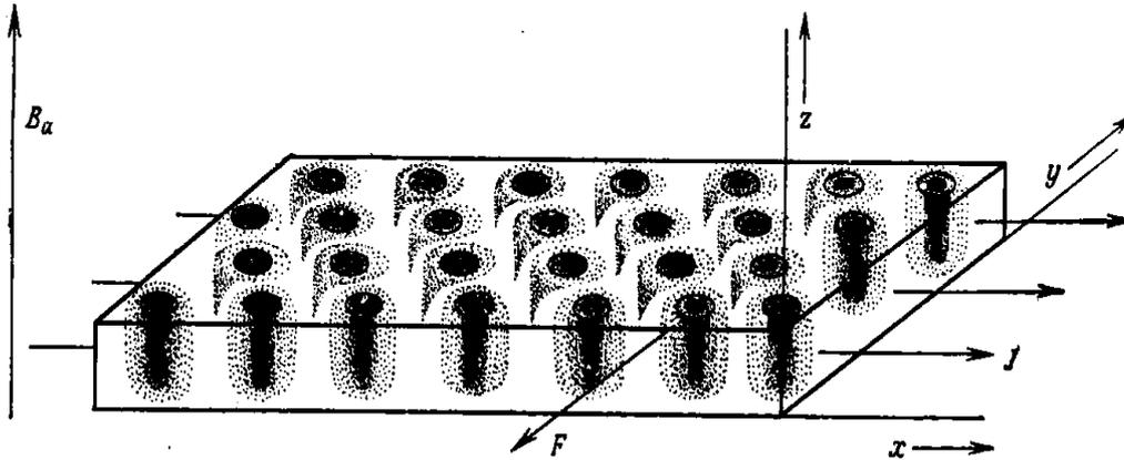
Figure 4.3. The mixed state in the presence of a transport current
