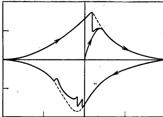
Fig.4.5. The entire cycle of magnetization.
