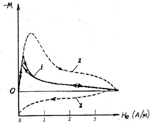
Fig. 4.4. Magnetization curve of an alloy  $Nb_{0.55}Ta_{0.45}$ : 1-a well-annealed sample, 2 – a sample with a large amount of defects.
